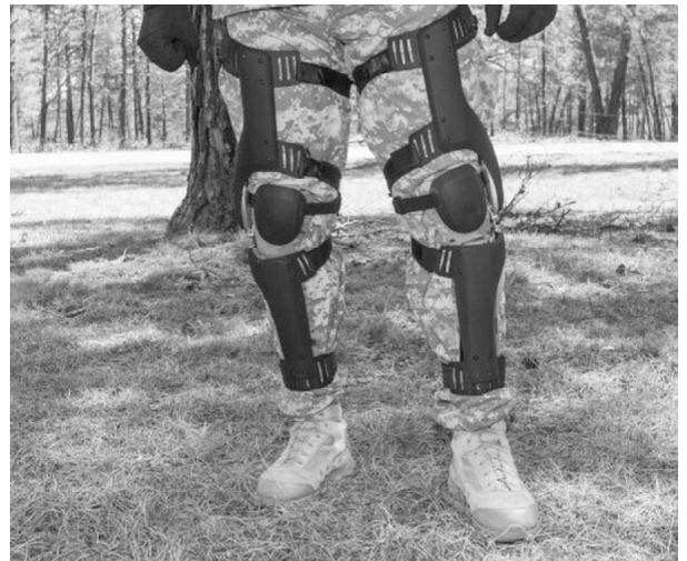
This unit uses knee motion to generate electricity
