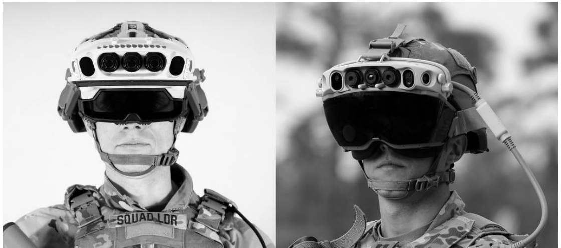
IVAS 1.2 (left) features a lower-profile Heads-Up-Display (HUD) than IVAS 1.0 (right), improving comfort and performance.
