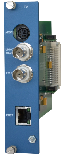
TW Circuit Board P/N: PCBTW-1-POP
