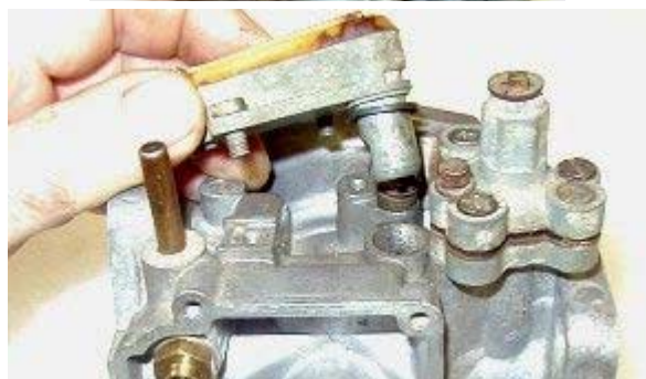
Removing the Temperature Compensator: one screw on each side and then pry out. Be sure to not lose the two fiber washers, one around the part that extends into the body and the other at the bottom of the hole in the body. These washers are not included in some rebuild kits.
