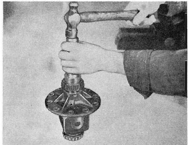
Fig. 27 Fitting differential bearings utilising the Churchill Tool No. M89 to the differential casing.
