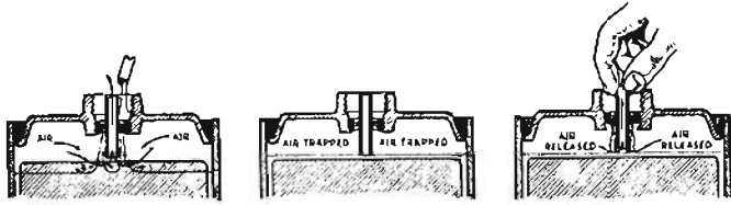
Fig. 1 Topping up Battery.
