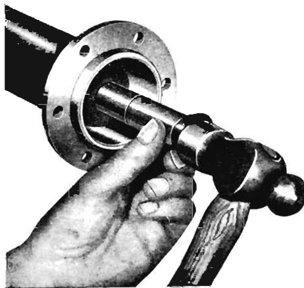
Fig. 8 Fitting oil seal into axle sleeve.
