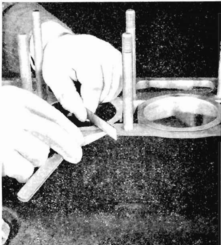
Fig. 5 Checking Cylinder Sleeve projection above Cylinder Block.
