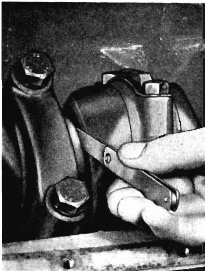
Fig. 17 Measuring Crankshaft End Float. This operation can be carried out with a Dial Test Indicator.
