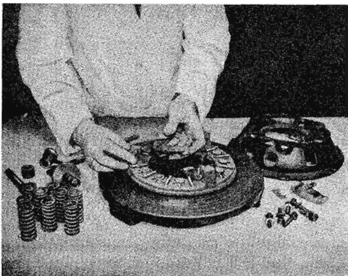
Fig. 11 Fitting Release Levers to Pressure Plate.
