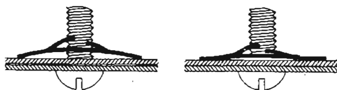
Fig. 3 Showing an Untightened Spire Nut on the left of the illustration and on the other side a fully tightened one.
