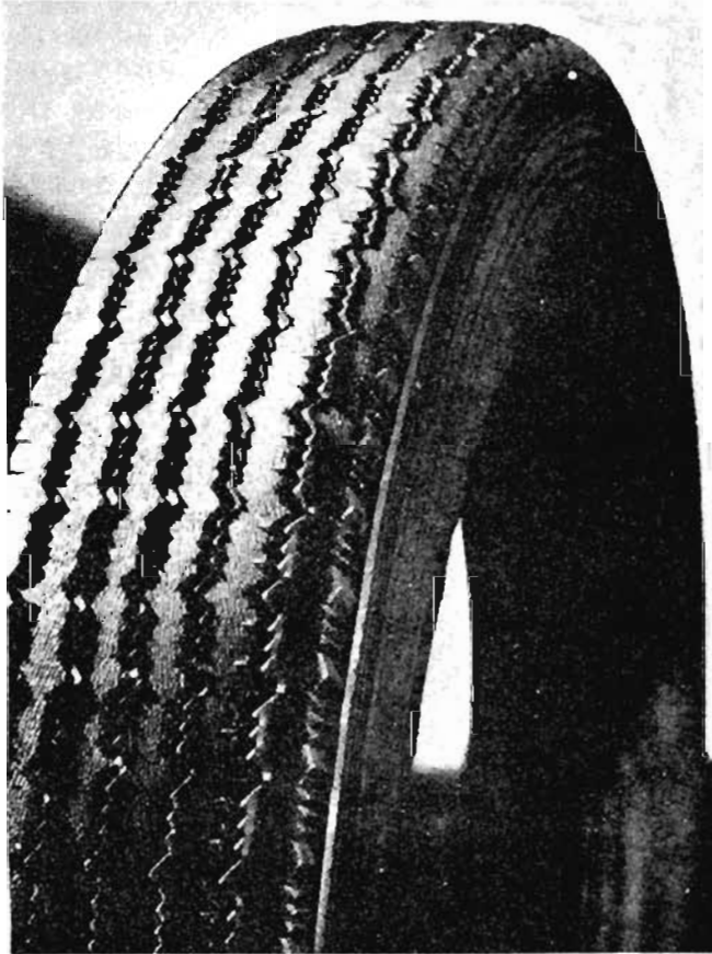
Fig. 12 Fins and Feathers due to severe misalignment.
