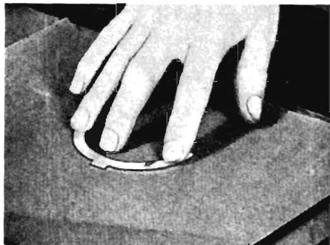
Fig. 18 Reducing the thickness of a Thrust Washer. This must only be carried out on the Steel Side.
