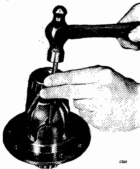
Fig. 84. Securing the cross shaft locking pin
