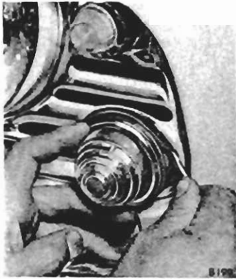
Fig. 28. Removing the lens from the direction indicator flashing lamp
