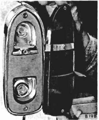
Fig. 30. Removing the lens from the tail, brake stop and direction indicator flashing lamp
