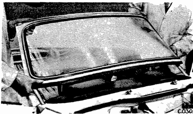
Fig. 12. Removing the windscreen
