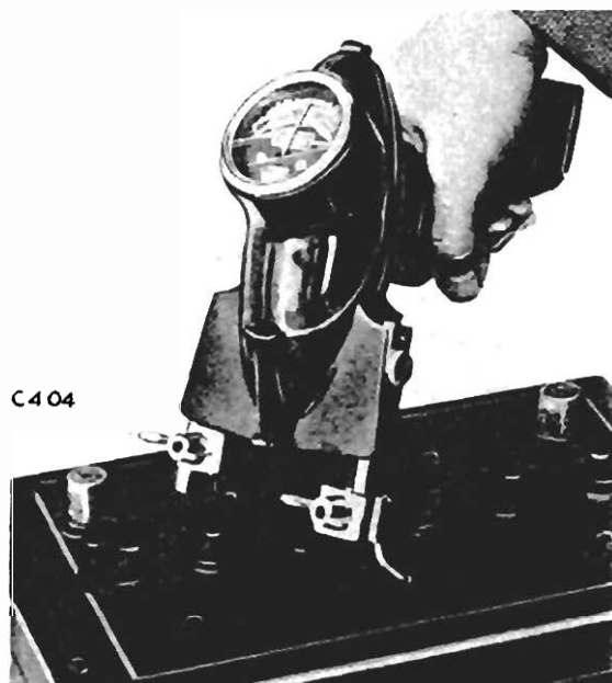
Fig. 6. Using a heavy discharge tester
