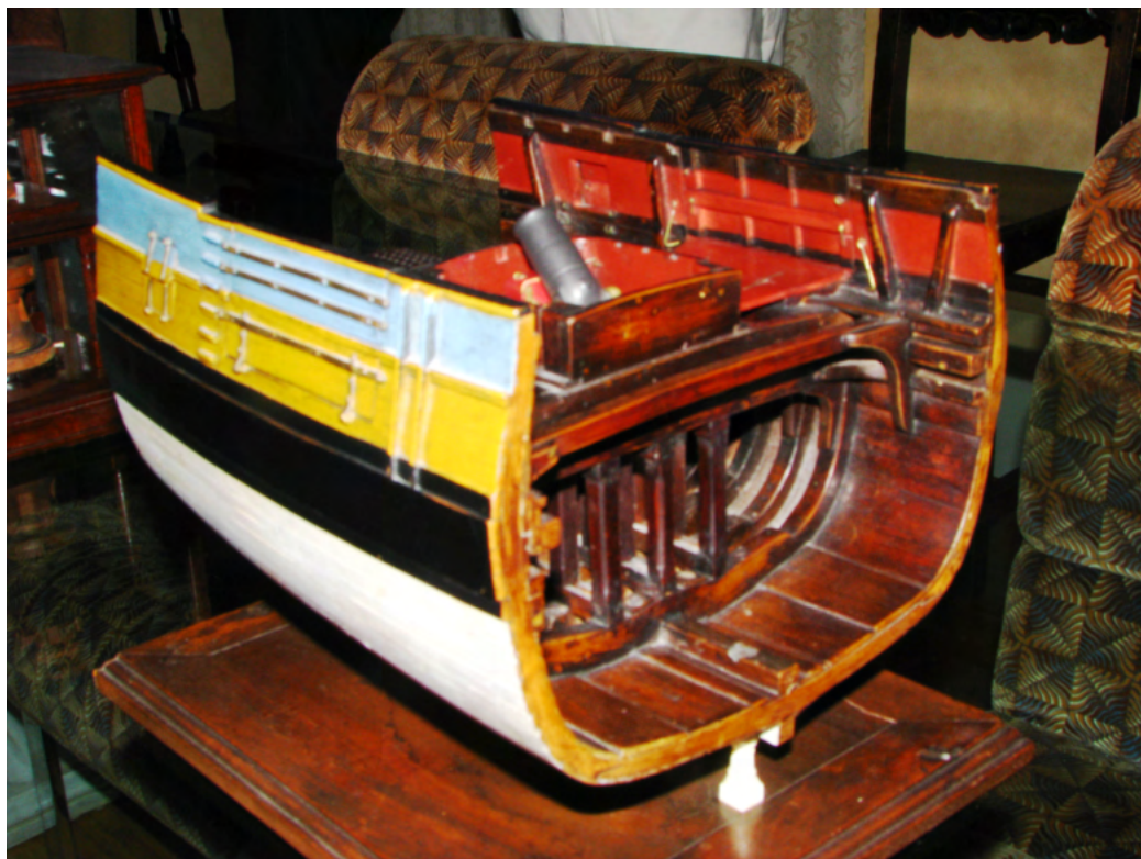
Fig. 13. Midships X-section of the Sulphur bomb vessel of 1797 showing the mortar supports below deck.
