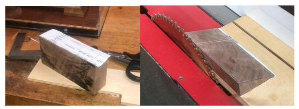
Fig. 8. Left-gluing piece of paper onto surface of small subject wood piece. Right-then gluing the small subject wood piece to a larger piece of  $\frac{1}{2}$ " plywood with the paper sandwiched in the glue joint and making the needed cut with your hands safely away from the saw blade.
