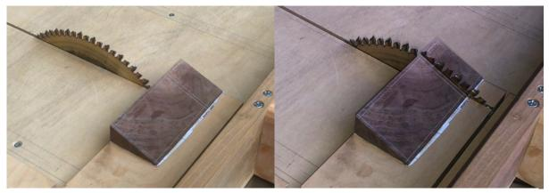
Fig.9. Cross-cuts can also be made in this way as well. It is done here on a cross-cut sled.
