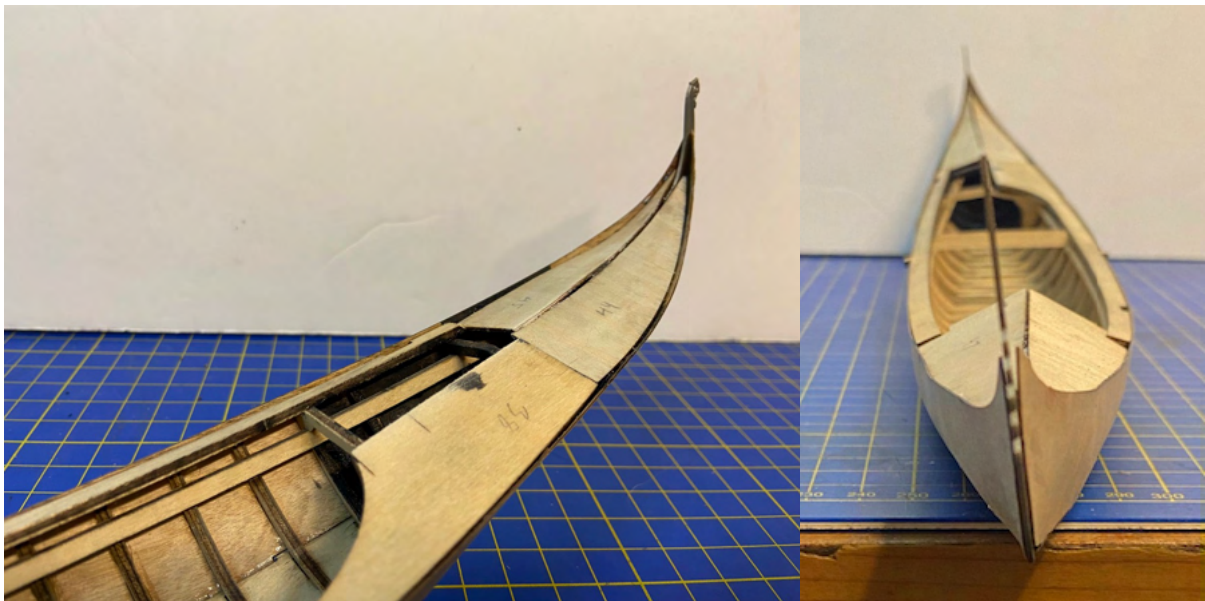
Fig. 11. Venetian Gondola Left -Close up of the partially completed bow. Right -The deliberate asymmetric form of the hull allowing the oarsman to row the boat only from the right side without having to switch the oar from side to side. . (Clare Hess)
