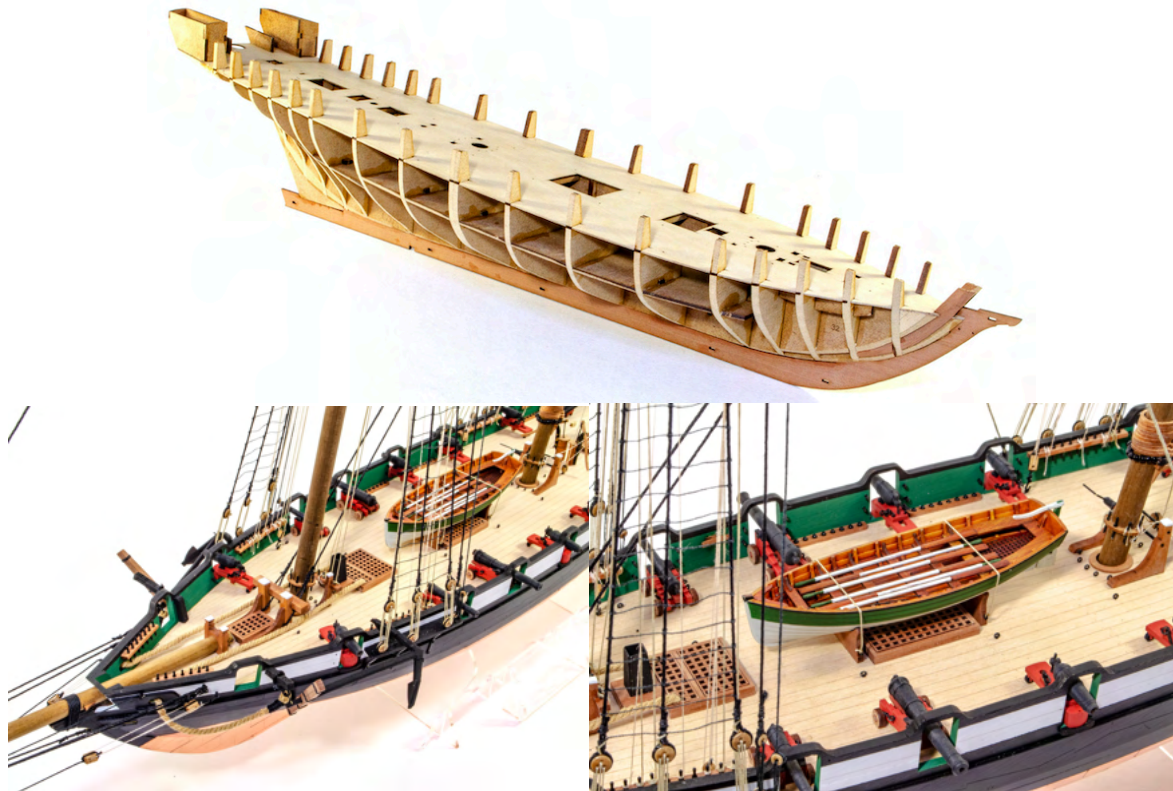
Fig. 8. Detail pictures of the frame (top), bow (lower left), and midships (lower right). (Vanguard Models)
