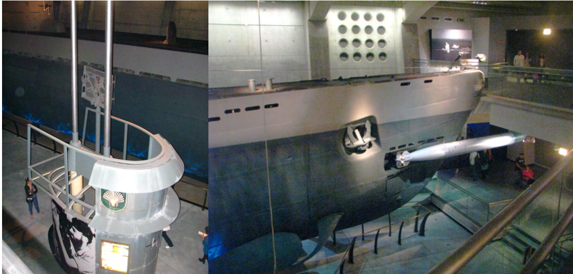
Fig. 22. Left-The submarine's periscope has been removed and remounted in a replica conning tower to improve public access to the instrument.
