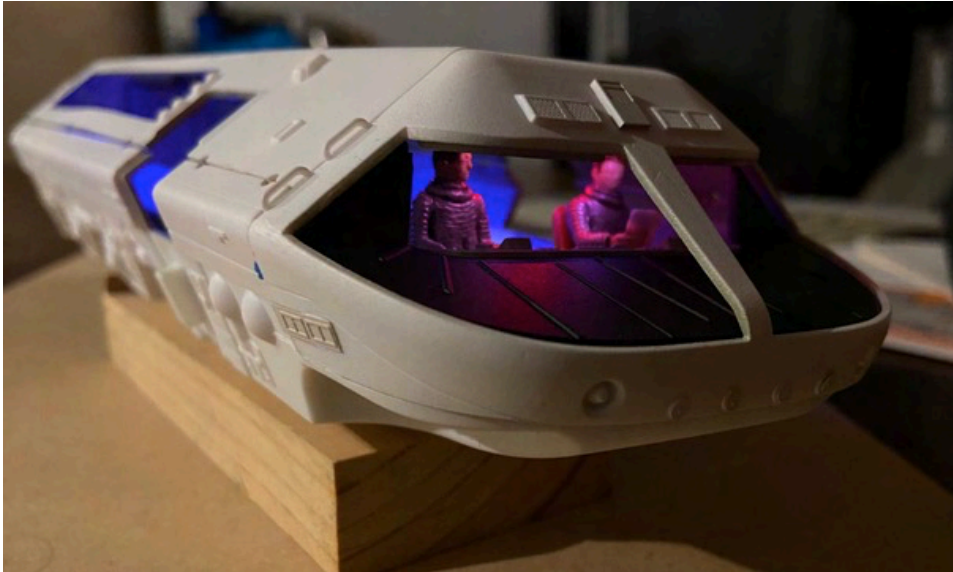
Fig. 6. LED lights illuminating the interior of a Moon Bus model from the movie, 2001: A Space Odyssey . The LED bulbs are not attached to any wires inside the model. Instead, the bulbs are powered wirelessly from an electrical induction coil installed in the base. There is no need to install wiring inside the model itself. (Clare Hess)
