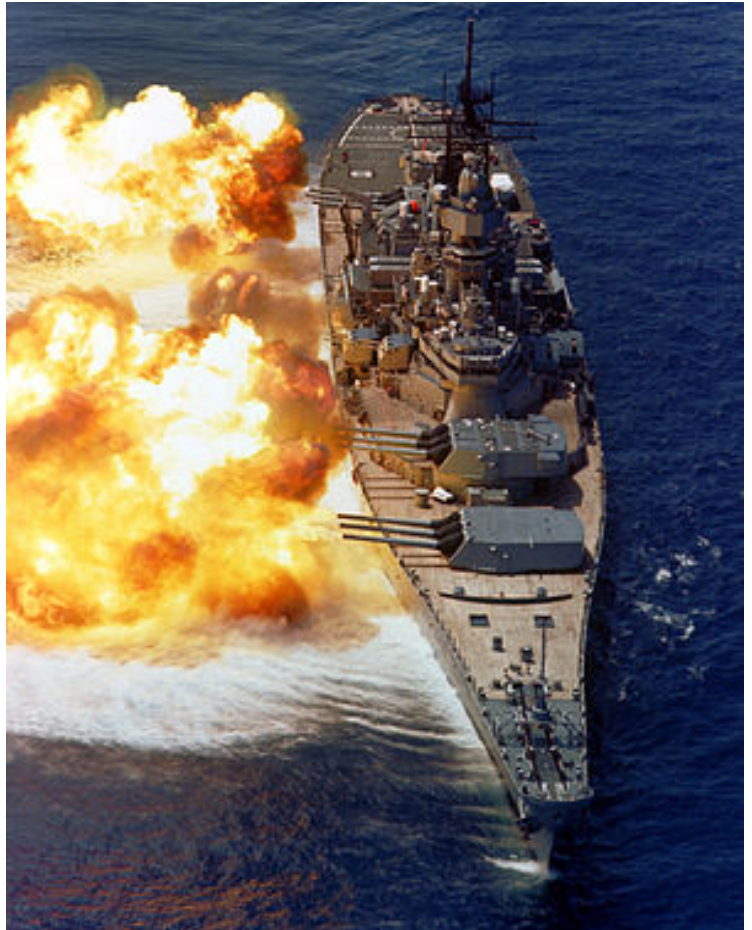
Fig. 5. BANG!! USS Iowa unleashes a broadsides of nine 16-inch guns on 15 August 1984 during a firepower demonstration
