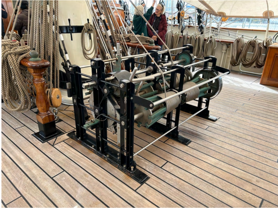
Fig. 9. Ship's winch behind the mainmast. Looks like it is operated manually by the crew. I did not see a motor mounted.
