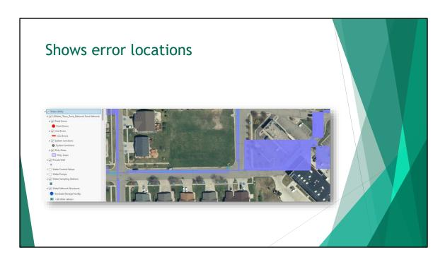
Image shows the trace network errors for points and dirty areas. Can be removed by validating on the trace network tab by either extent or entire dataset.
