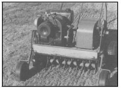
Figure 11. Vertical mower.
