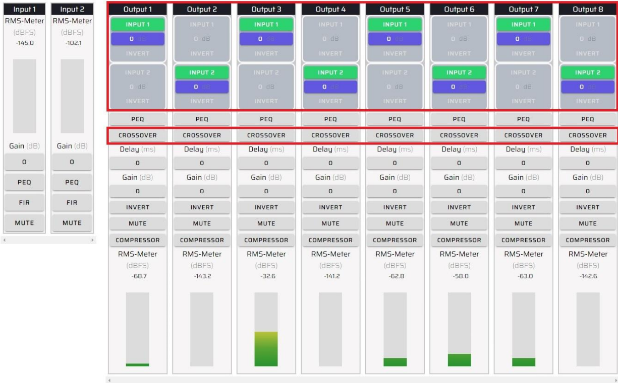
Diagram 2. Crossover speaker selection and parameters are modified in the areas highlighted in red
