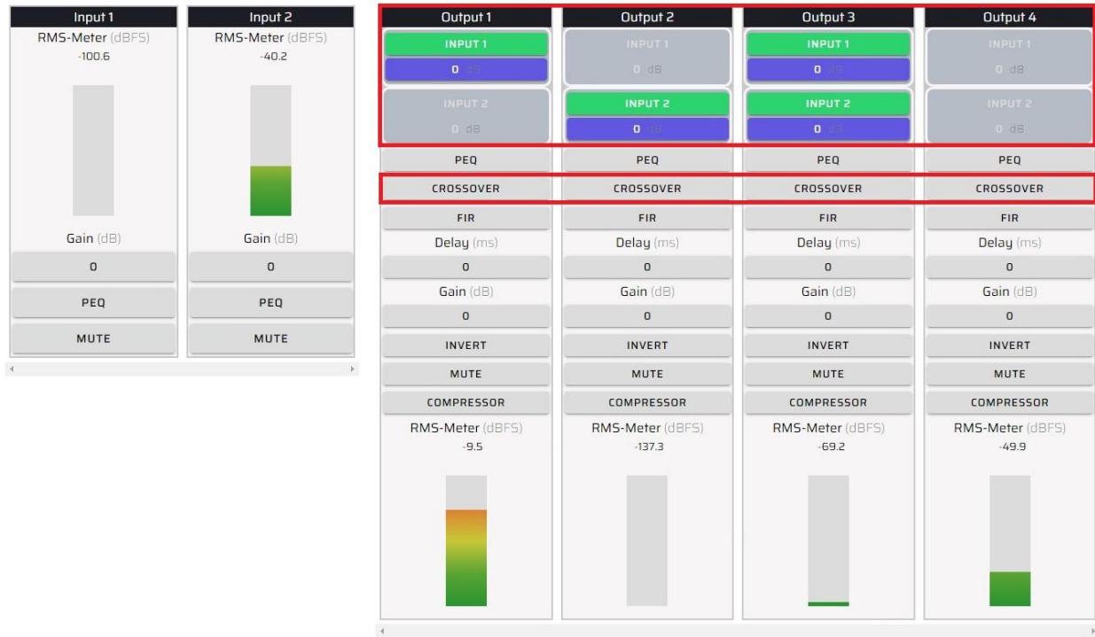
Diagram 10. Crossover speaker selection and parameters are modified in the areas highlighted in red
