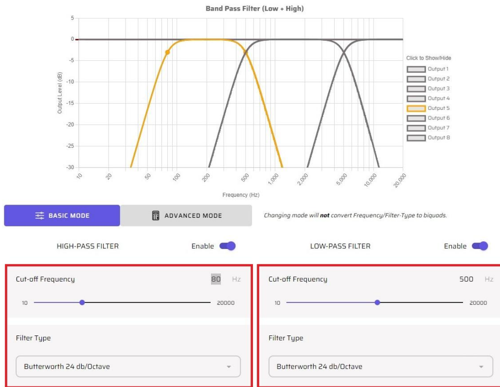
Diagram 7. Woofer band pass filter
