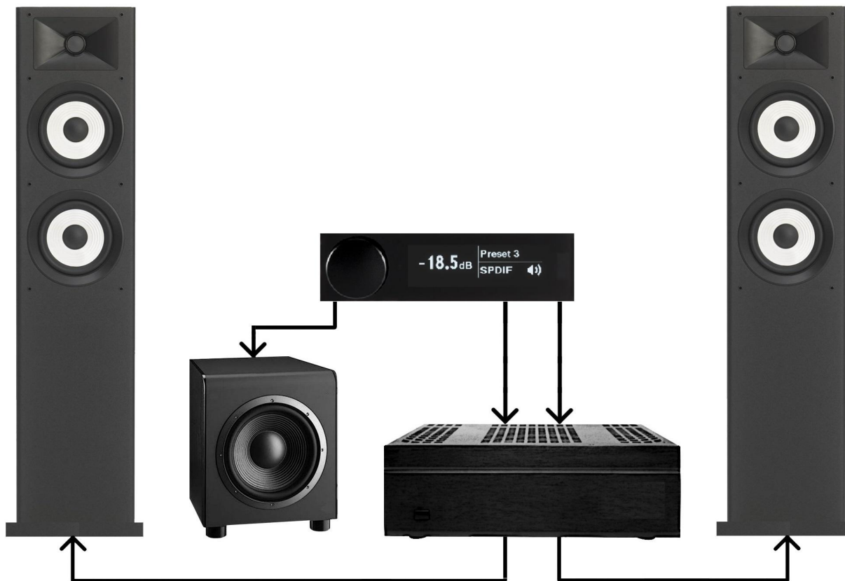
Diagram 9. Active subwoofer 2.1 stereo system
