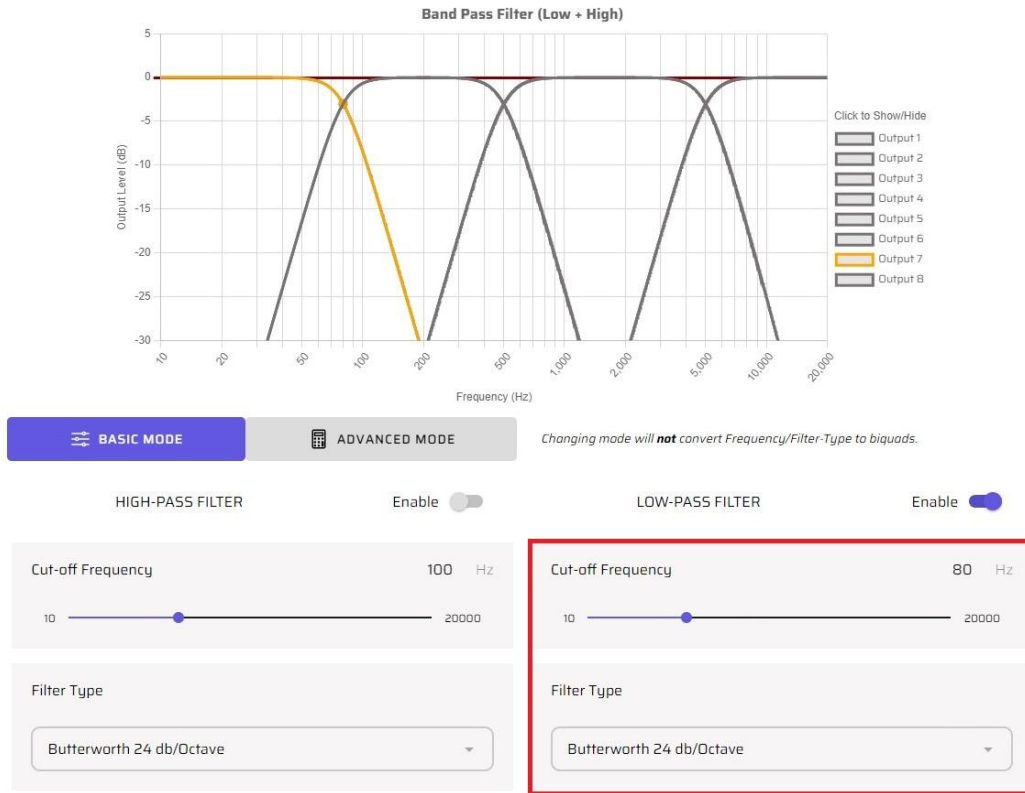
Diagram 8. Completed active speaker four-way crossover
