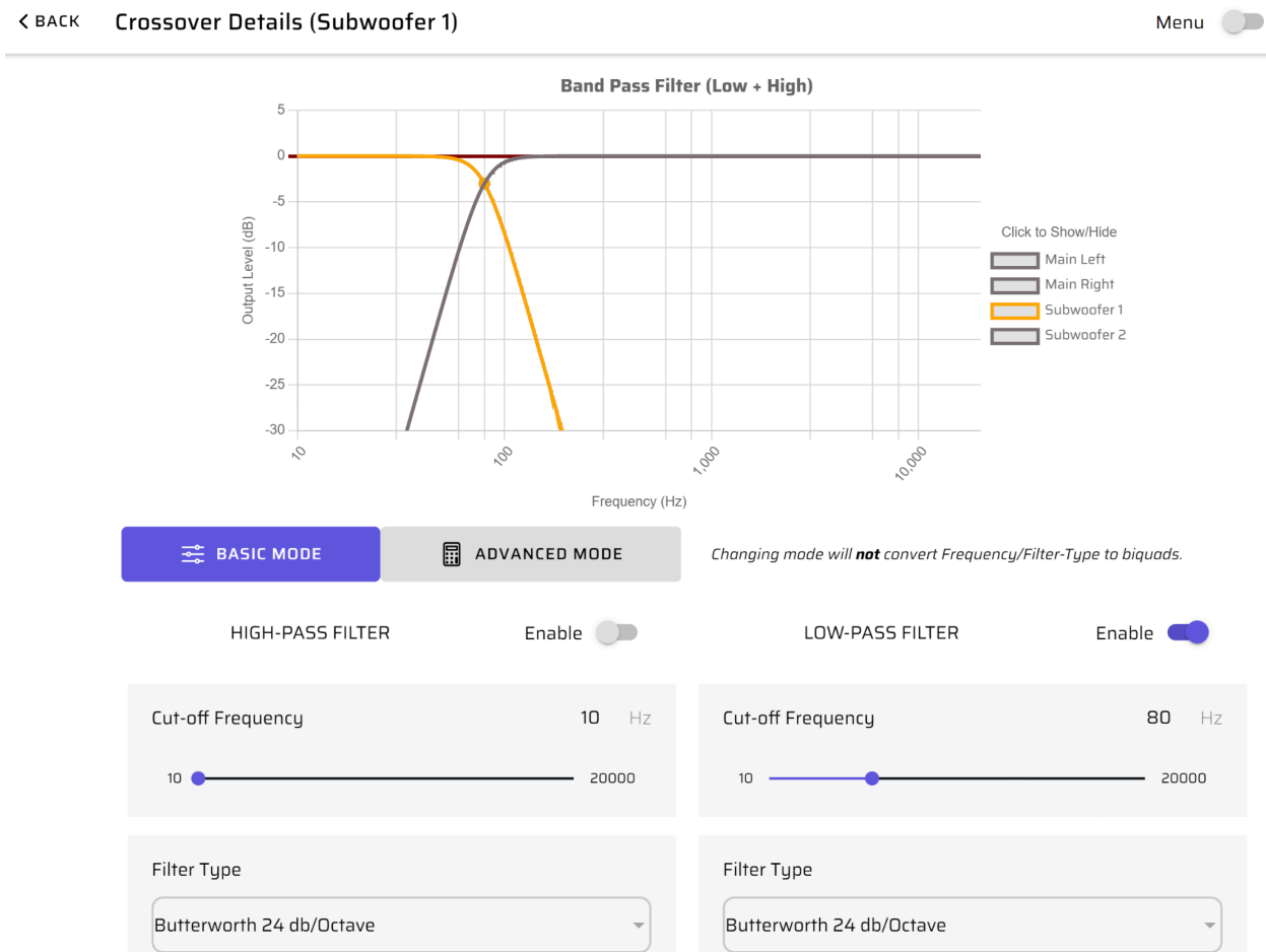
Diagram 7. Example of a classic Butterworth symmetrical crossover
