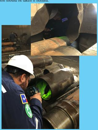
WET MAGNETIC PARTICLE INSPECTION
