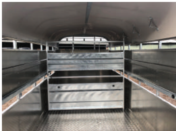
Additional dividing gate.
