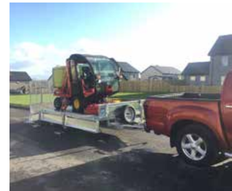
Can load pallets with forklift from the side using removable drop sides
