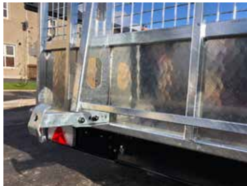
Fully integrated prop stands offer loading support, stability and are adjustable to suit ground types
