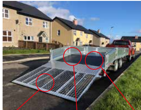
Full width ramp tail door allows loading of machinery of various widths and wheels
