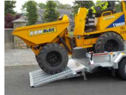
Low centre of gravity with a bed height of 403mm, giving a favourable loading angle, which is great for equipment with low ground clearance
