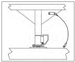
Breakaway Brake Lanyard - Figure 4-10.
