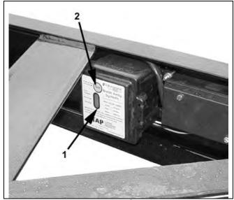
Breakaway Brake Battery Charger – Figure 4-4
