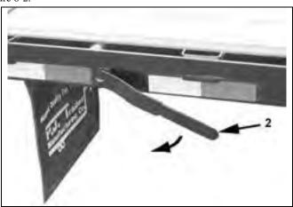
Dovetail Mechanical Stop Handle - Figure 6-3
