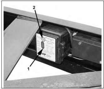
Breakaway Brake Battery Charger - Figure 4-9
