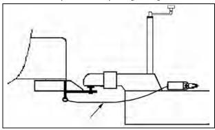
Breakaway Brake Lanyard – Figure 4-5
