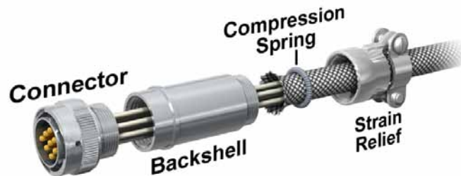
Figure 2. Compression Spring Backshell Assembly
