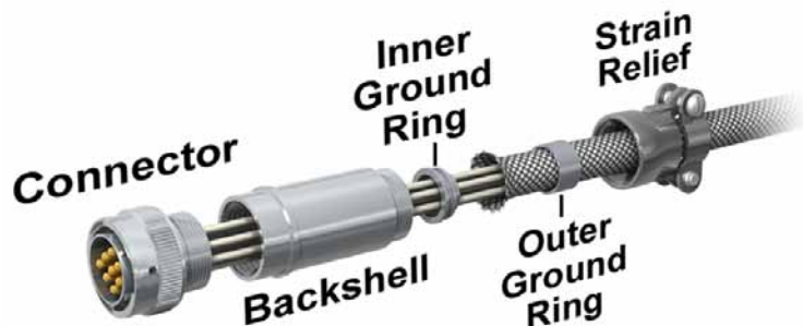
Figure 1. Typical Cone and Ring Backshell Assembly.
