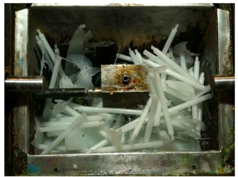
MOLDVILLE is the ultimate recycling machine. What doesn't get put into the Club-A-Rama, ends up back in the vat to be remelted into the next week's figure! Here you see mostly the discarded evacuation tubes from the Space Needle production.
