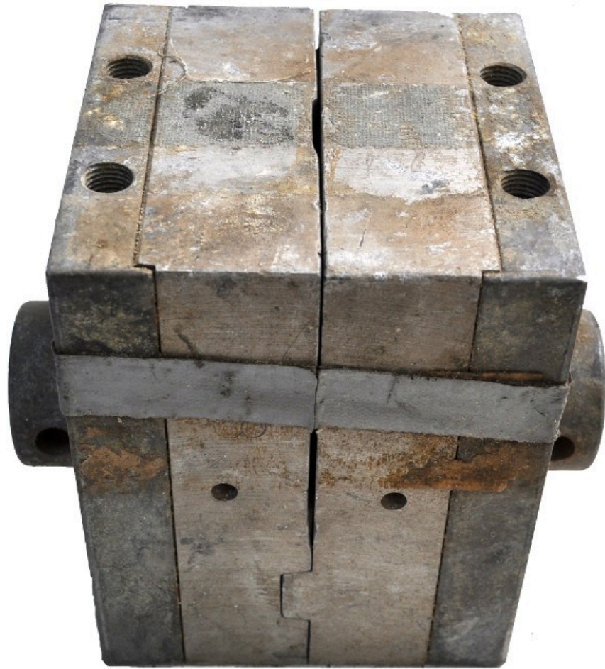
Each half of these extremely early milled moldsets are made of a solid block of aluminum, and cooled from the back with a back plate that has a "U" shaped cooling path drilled through it. (See the entrance and exit tapped holes at the top of each back plate?) Needless to say, this minimal cooling design is not nearly as efficient as later designs that run chilled water directly through each hollowed cast mold half.
