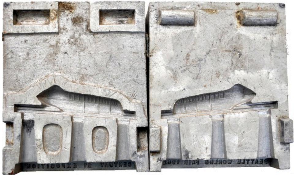
The Alweg MONORAIL from the 1962 Seattle Worlds Fair is yet another one-of-a-kind, only-one-ever-made, historic mold used by MOLDVILLE.com to reissue this week's souvenir figure for the Club-A-Rama! The Alweg MONORAIL appears to be a milled mold (not cast) and exhibits an early mating design that was soon changed for production moldsets.
