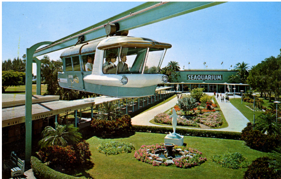
Constructed in 1963, the Miami Seaquarium Monorail was billed as the first of its kind on the East Coast. Suspended on a 2385 foot long guideway, five cars (with one in reserve) carried guests on a 6 mph trip past show and exhibit buildings. The original cars were each named for a fish and had operating headlights and air conditioning.
