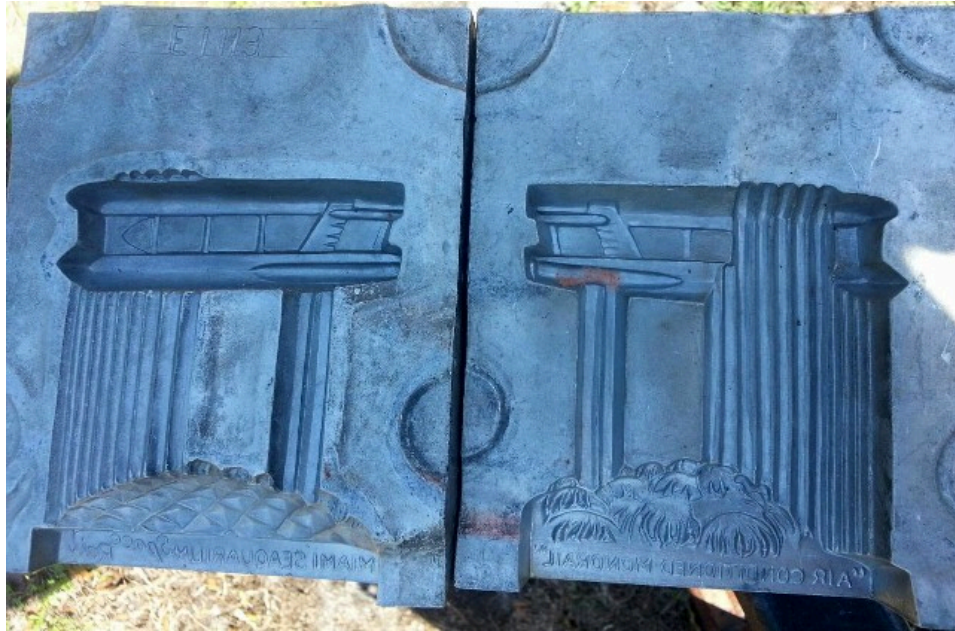
The Miami Seaquarium SPACE RAIL moldset, numbered 1113, was a custom moldset made in 1964 for use at the Miami Seaquarium.
