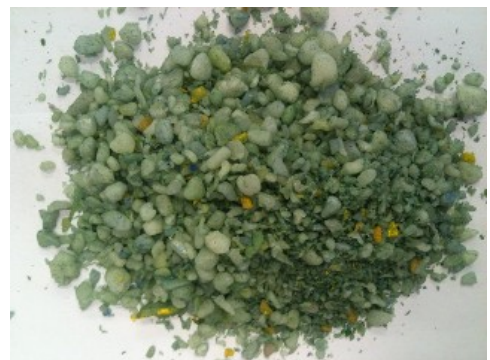
This is what the final Moldville RetroWax™ product looks like after the ingredients are professionally mixed, melted, hardened, and ground. It looks VERY similar in size and shape to original wax samples we've been able to recover from old machines:
