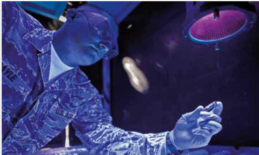
NDI Technician of the 22nd Maintenance Squadron dips a section of a KC-135 Strato-tanker's landing gear in fluorescent chemicals and inspects using a Labino UVG3 2.0 UV light at McConnell Air Force Base.
