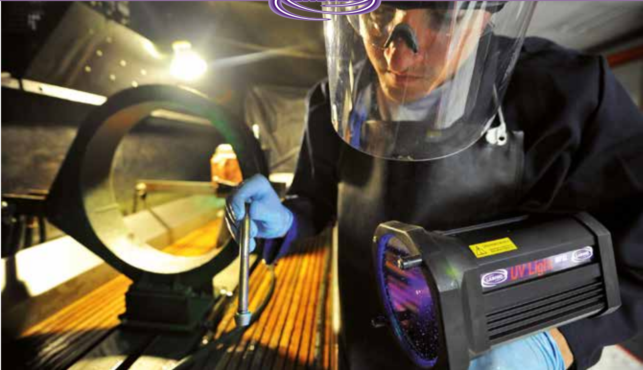
NDI Technician of the 86th Maintenance Squadron takes a closer look at a nose landing gear wheel bolt during a magnetic particle inspection at Ramstein Air Base, Germany.
