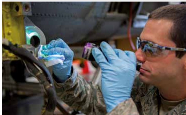
NDT Technician of the 18th Equipment Maintenance Squadron checks for cracks and chips that could lead to a structural failure during a phase inspection at Kadena Air Base, Japan.
