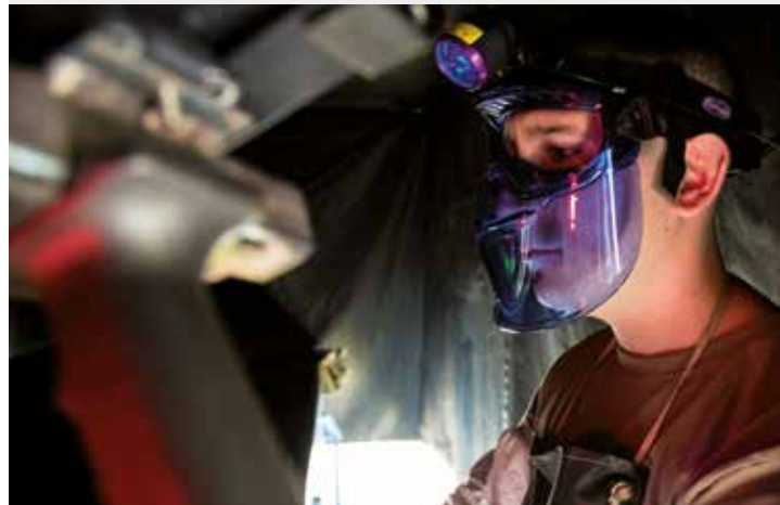
NDI Technician of the 108th Maintenance Squadron, analyzes a part of the KC-135R Stratotanker aircraft at Joint Base McGuire-Dix-Lakehurst, N.J., using a Labino UVG5 headlight.
