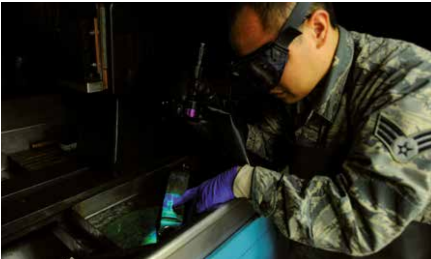
NDI Technician of the 22nd Maintenance Squadron dips a section of a KC-135 Strato-tanker's landing gear in fluorescent chemicals and inspects using a Labino UVG3 2.0 UV light at McConnell Air Force Base.
