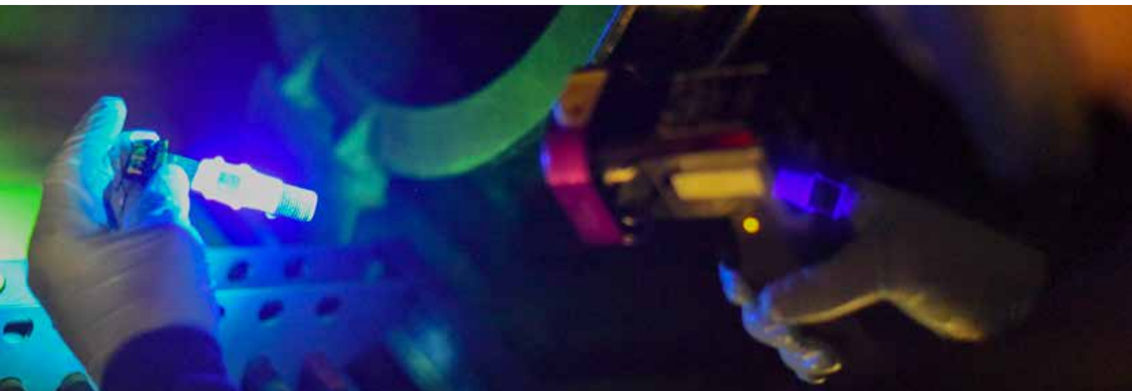
NDI Technicians of the 100th Maintenance Squadron perform a magnetic particle inspection on sample parts, at RAF Mildenhall, England, using Labino MB 2.0 Series UV lights.
