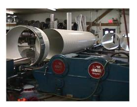
Spiral Pipe can be supplied in diameters from **3**" to **76**" in gauges from **26** Gauge to **14** Gauge. Spiral pipe can be supplied in lengths from 1 foot to 20 feet long.
