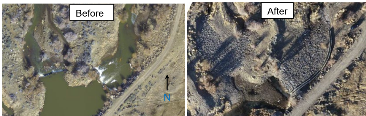
Figure 2. Before and after aerial photos of the Starveout diversion showing rock ramps on east and west channel. The PIT antenna was installed only on east channel that receives most of the streamflow.
