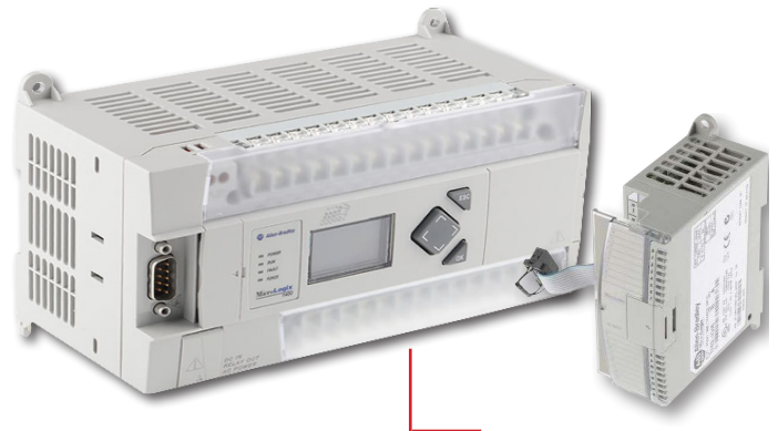
Allen Bradley Micrologix 1400 processor, 1766-L32BWAA with 16PT input module 1762-IQ16
