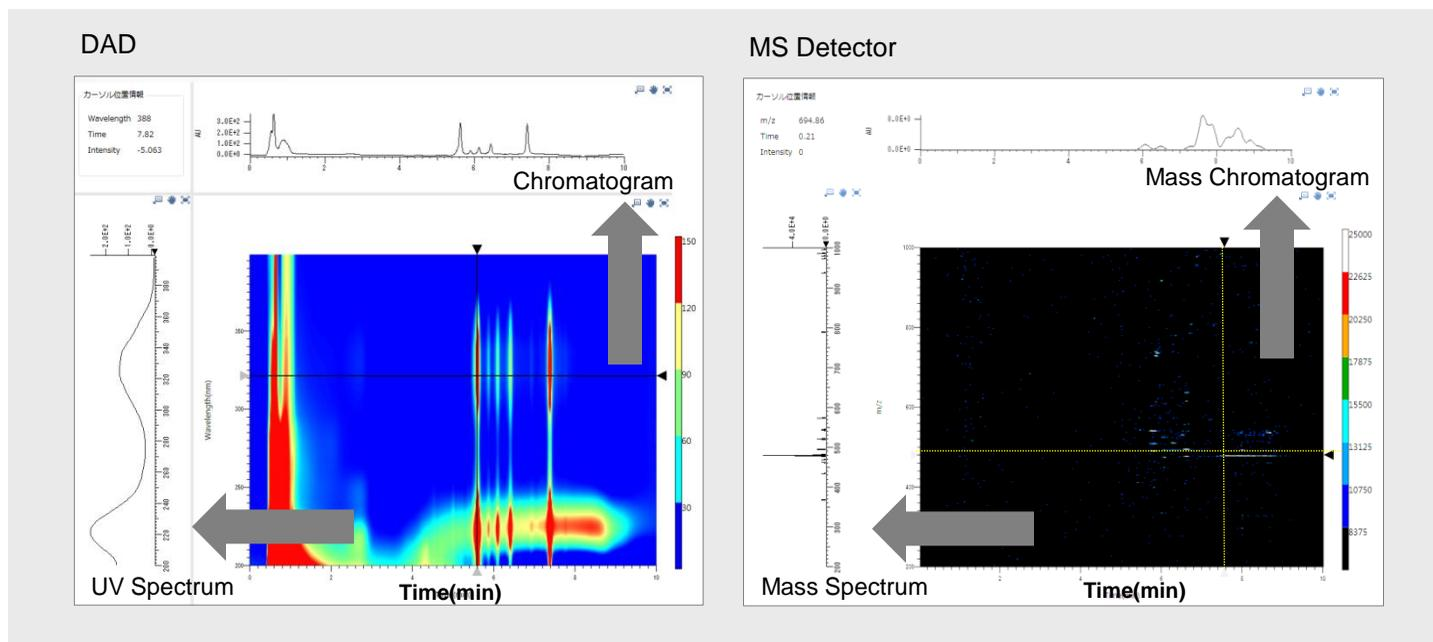
Figure 1 Contour Plot Based on DAD and MS Scan Analysis Results
