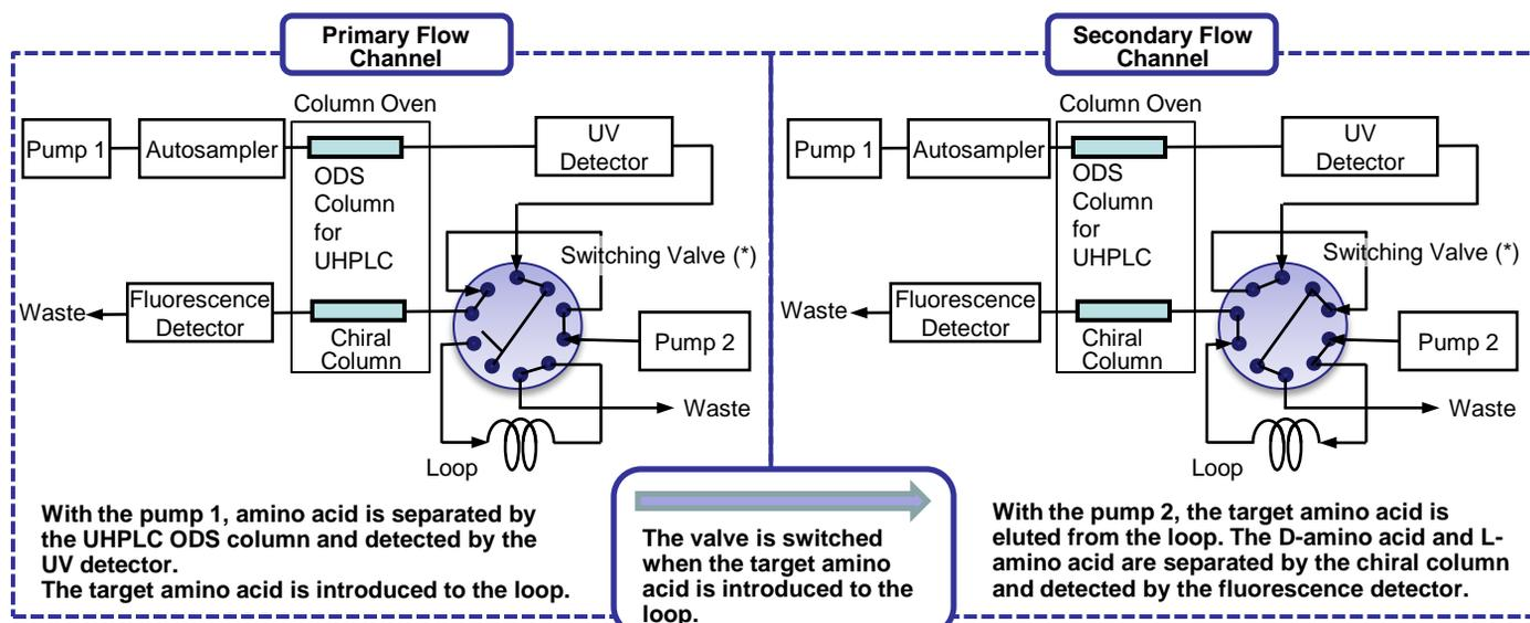
(\*) While a 10-way switching valve was used this time, a 6-way switching valve can also be used.
