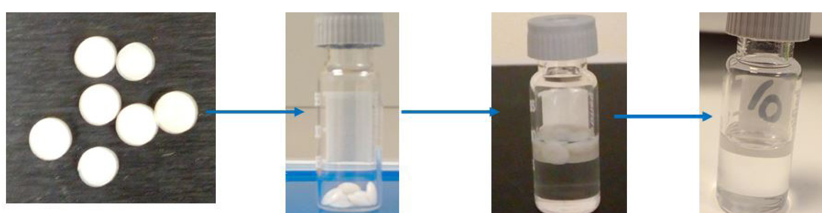
Figure 1. A simple solvent extraction of limonene from HDPE
