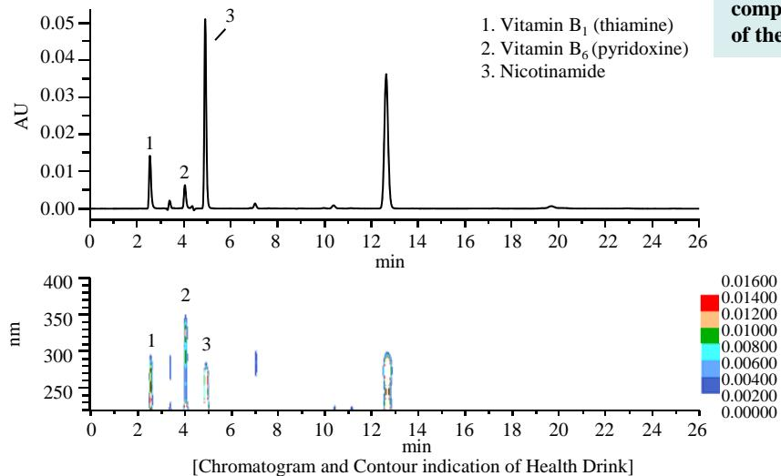
By using DAD, detected peaks can be identified from comparing the absorption spectrum with the spectrum of the standard.
