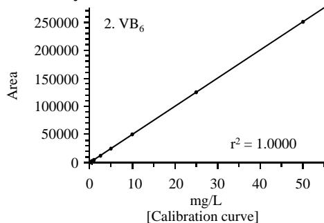
All of the calibration curves (all components in the range from 0.1 to 50 mg/L) exhibited high linearity, with  $r^2 = 0.996$  or more. However, Vitamin C, Erythorbic acid, and Vitamin B<sub>12</sub> are unstable when diluted by this eluent. It is important to use fresh sample for obtaining good linearity. Please note this procedure should be used mainly for qualitative purposes.
