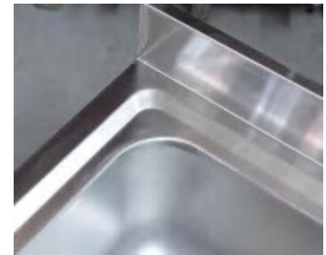
Nice polishing finish after welding
