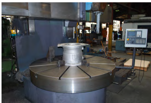
DN350 NCV- BODY SEAT MACHINING
