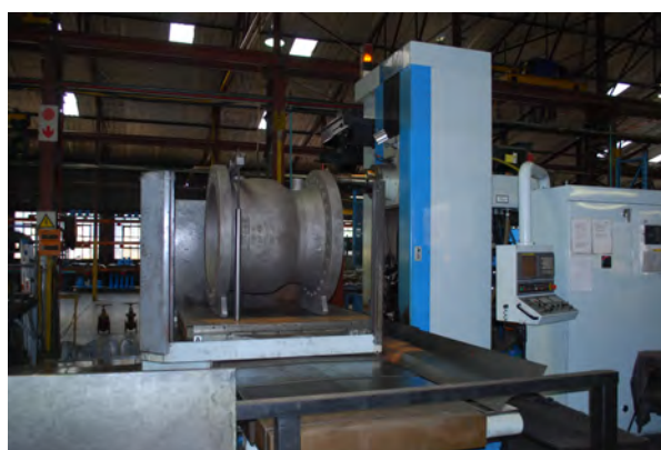
DN900 (36") PN25 NCV-B FLANGE MACHINING
