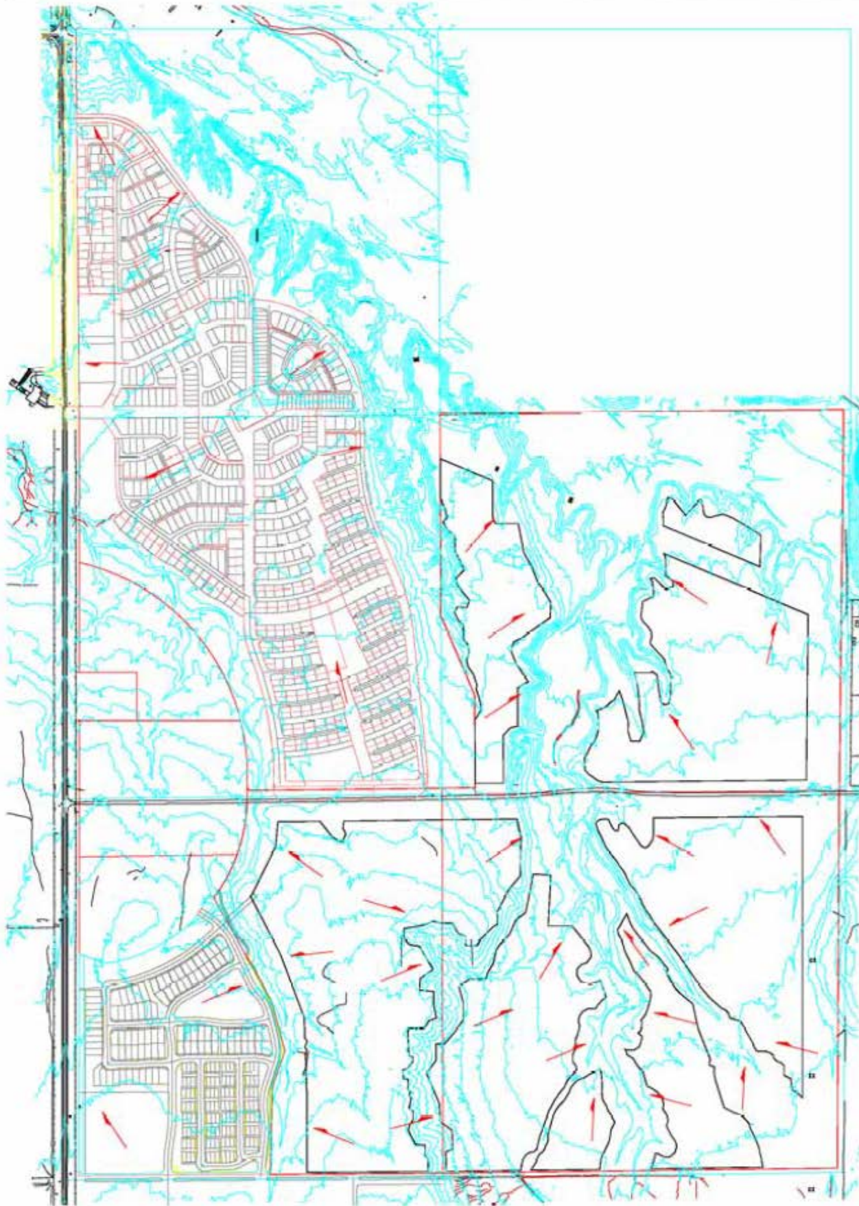
FIGURE 18: POST DEVELOPMENT HYDROLOGY
