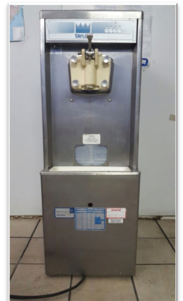
An example of a single flavor soft-serve machine.
