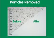
Oil cleanliness maintained at better than new levels (Down to 13/11/8 (ISO 4406: 1999) - Class 2 (NAS 1638).
