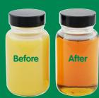
Removes free and dissolved water down to < 50 ppm (0.005%)
