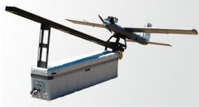
Device used to launch a fixed-wing Air Vehicle from the ground. The details of this option include the following:
