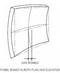
A problem encountered in the field is that convex bowing cannot be measured as shown after the stone has been installed. To measure convex bowing after installation, shims and a straight edge are employed.
