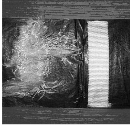
Figure 1. Untreated (left) and Insecta™ RXT treated (right) PA sheets after 1 week of rodent exposure. The untreated were damaged fully by gnawing.
