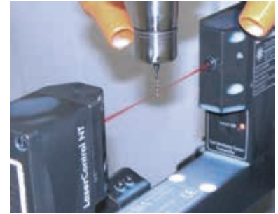
Support systems provide highest precision even with micro-tools
