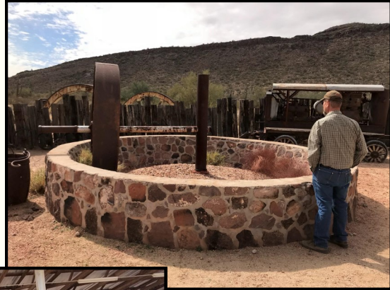
An arrastra -- ore is crushed, as horses or mules pull the heavy around and around...
