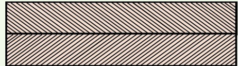
FIGURE 3 Herringbone Crossbeds Where the current reverses frequently, such as in tidal area, zig zag crossbeds, called herringbone crossbeds, form.
