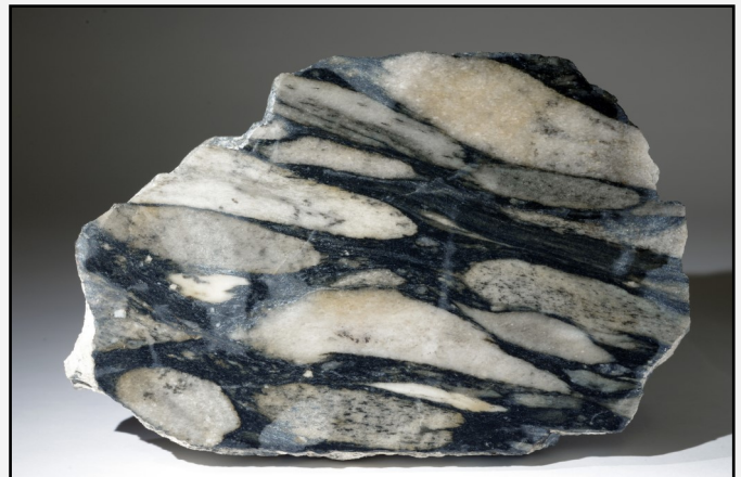
FIGURE 14 This metaconglomerate has been sawn, exposing the intimacy of the pebble/matrix boundary -- this is a very dense rock. (Enlarge the view for a closer look!) Photo by Stan Celestian
