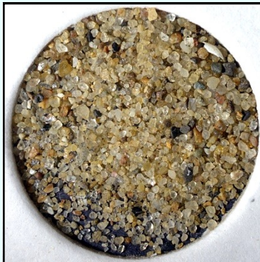
FIGURE 8 Fluvial Sand — a River Sand Bar at Falls of the Ohio, IN This sand reflects a lot of weathering and transportation — angular to rounded quartz grains, with few of other minerals. Stream sands will generally have a varied range of sand sizes.
