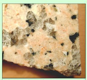
FIGURE 14 Coarse Granite This polished fragment of granite countertop clearly reveals fairly large crystals of gray granite, pink feldspar, and black biotite.
