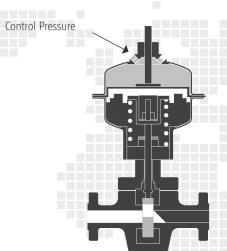
Upon application of adequate control pressure to the actuator, valve begins to open (gate moves down)
