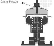
Upon loss of control pressure, valve begins to close (gate moves up)
