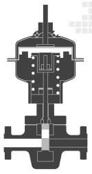
Valve fully closes and remains closed until application of control pressure to the actuator (gate all the way up)
