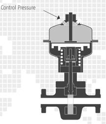
With continued application of adequate control pressure, valve moves to the fully open position (gate all the way down)
