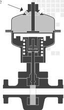
Valve remains in fully open position as long as adequate control pressure is present (gate all the way down)
