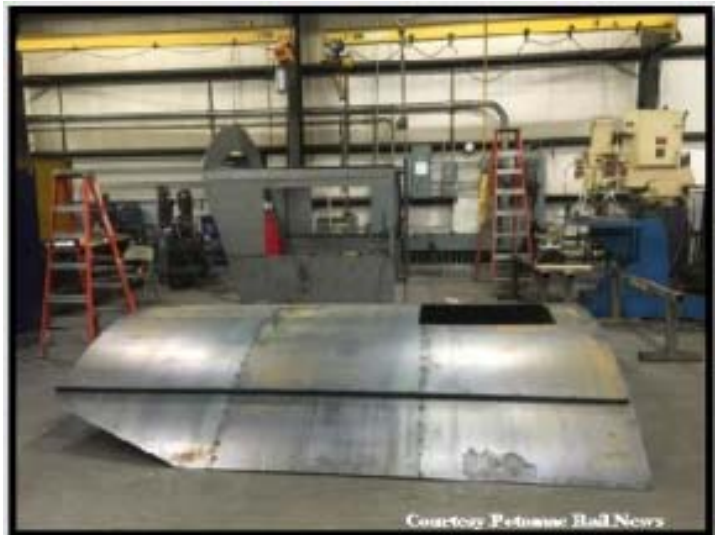
New cab roof with the new cab in the background.
