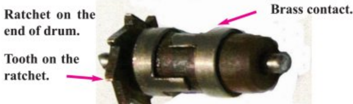
Fig. 2. The Ives R-unit drum has a ratchet with teeth pressed on one end. The pawl catches a tooth and rotates the drum. The brass contacts on the drum rub against two sets of copper fingers
